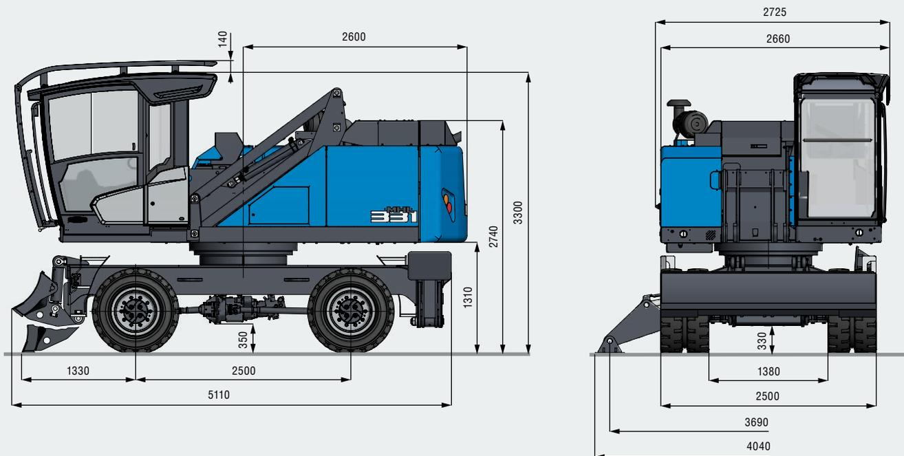
**TRANSPORT DIMENSIONS | TRANSPORTABMESSUNGEN | DIMENSIONS DE TRANSPORT [mm]**
