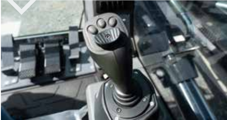
ELECTRIC JOYSTICKS are fully adjustable to accommodate the preferences of each operator. Additionally, three different joystick variants are available.
