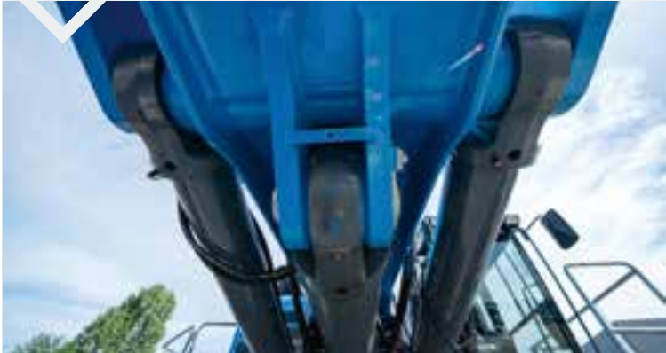
DUAL-EAR PIN CONNECTION OF BOOM & STICK ensures optimal force distribution, reduced wear through lower stress, and offers outstanding durability.
