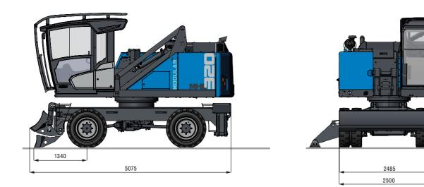
**TRANSPORT DIMENSIONS** Side view all dimensions in mm FUCHS 2920 11475 12800 **8.2** m \*\* **9.2** m\*\* 7545 mm 8625 mm А 3480 mm 4140 mm В 3150 mm 2850 mm С
