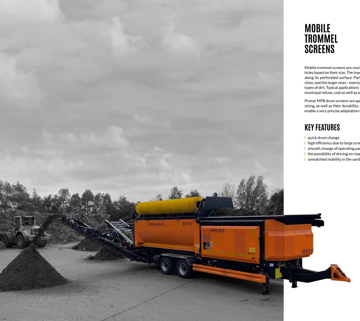
Mobile trommel screens are machines whose task is to mechanically divide particles based on their size. The input material falling into the rotating drum moves along its perforated surface. Particles smaller than the mesh form the fine fraction, and the larger ones - oversize. As a result, the material is cleaned of various types of dirt. Typical applications for drum screens are compost, wood chips, soil, municipal refuse, coal as well as aggregate.
